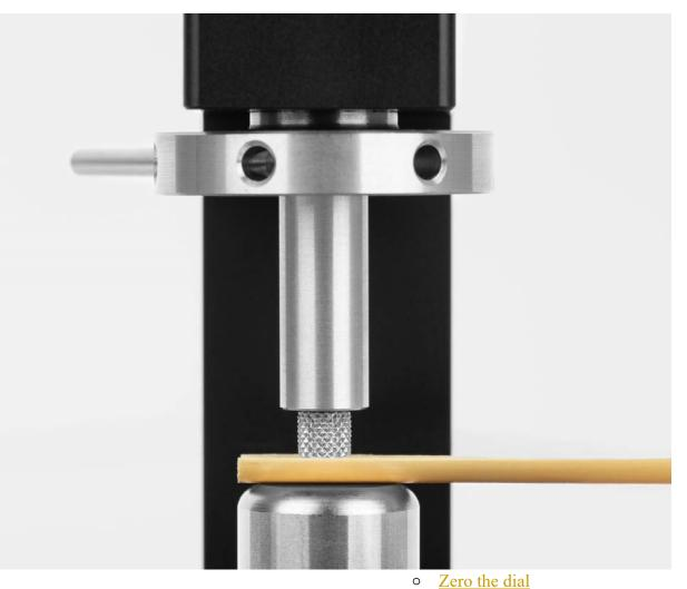
Turn the rotating handle from the right side to the **left** side of the hardness tester.
