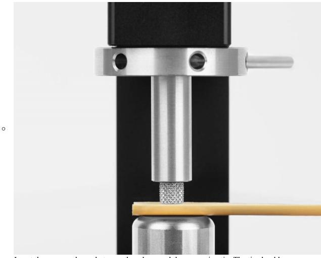
Insert the cane as shown between the arbour and the measuring tip. The tip should be about 1 cm from the end of the cane. The rotating handle should be on the **right** side of the hardness tester
