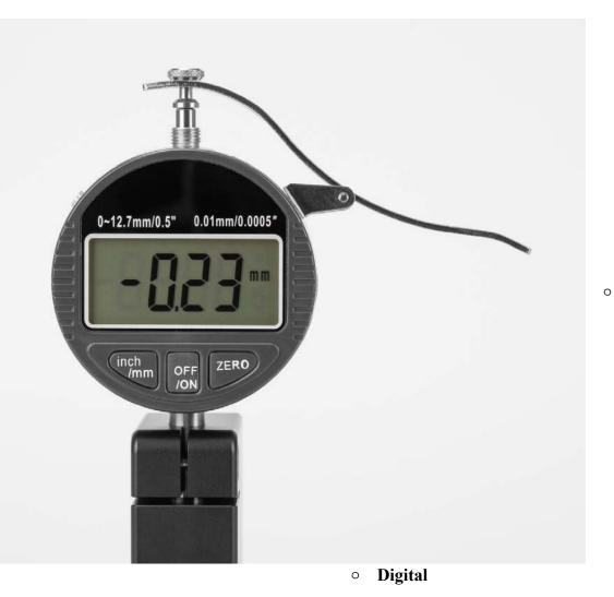
The readout will now read the hardness of the cane. You can ignore the negative as well as the decimal.
