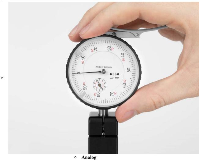
Rotate the dial so it is reading "0."
